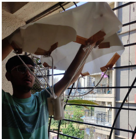
Figure 14: (I) Parachute Made Using Polyester Material of 20 Inches in Diameter (II) Parachute Attached To the Lower Stage of the Rocket
