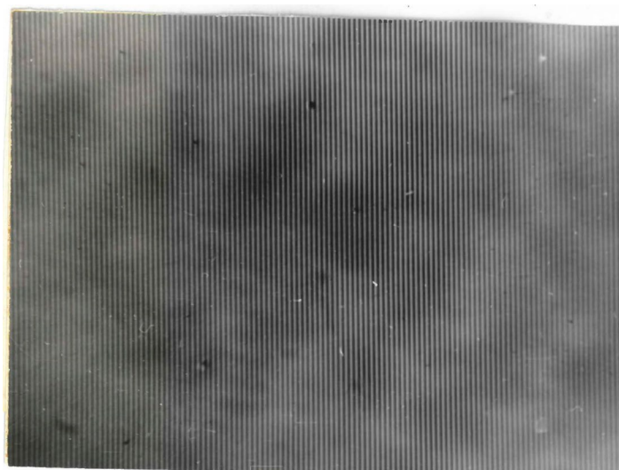
Figure 3: Is the Result of Interference of Two Flat Intersecting Laser Beams Recorded on a Photographic Plate
