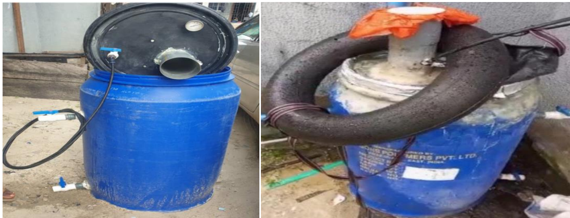
Figure 2: Photograph of Fabricated Mini Digester (Bioreactor)
