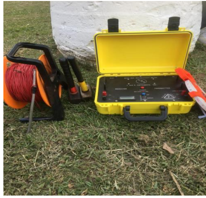
Figure 4: Mini-Res Resistivity Meter with Accessories
