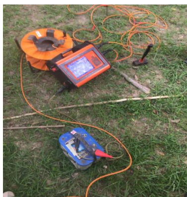
Figure 3: ABEM Terrameter LS with Accessories
