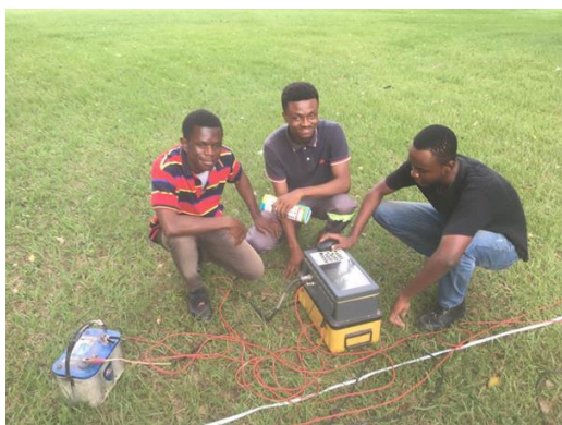
Figure 2: The SmartSeis Seismograph for Seismic Refraction Survey
