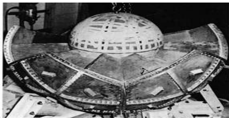
Same Y-1222 implosion design with six of the 12 large hexagonal Dural external sphere plates hoisted in place over the HE blocks. The 1/2" cork lining is visible on the inner surface of the Dural sphere along with the tape used to hold the felt covering in place over the 24.5" aluminum pusher-sphere. Since this was an early test unit, no detonator holes were drilled into the Dural sphere. The same 72-block non-leak design with the 24.3" pit was also used in the later Y-1291 model, which ultimately utilized the Y-1561 Dural case. (LANL/Courtesy of James Kuratka)
