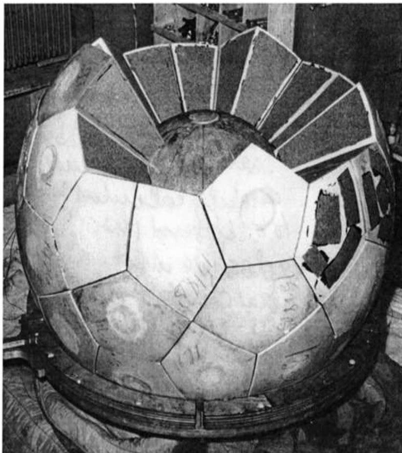
The 72-block Y-1222 implosion design showing blotter paper-faced solid Comp B non-lens HE blocks and 24.5" diameter felt-covered aluminum pusher sphere. Note the use of both regular and irregular pentagonal shaped charges in this design. No detonator holes were used in this test unit. (Courtesy of James Lyons, Sr.)
