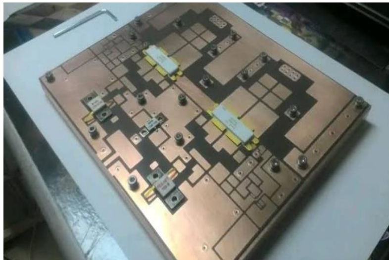
Figure 7: Photo of construction of class-D power amplifier
