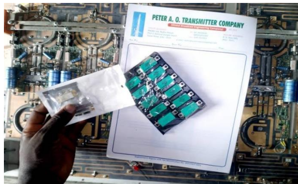
Figure 2: Photo of RF modules for amplitude modulation
